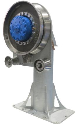
24" Stainless Steel or Manganese Bronze sheaves are adjustable with shims for use with 5/8" to 1-1/4" size line.
